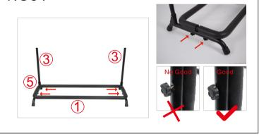
4. The tube with most holes of No2 need to put on the bracket of NO3. and the connection has a fixed interface correspond to the spring button, which can be stuck by pressing it with the fingers.
