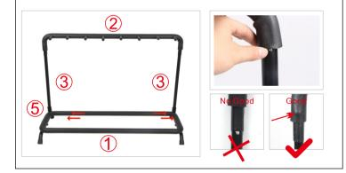
5.Put all the accessories of No4 to install on the tube of No3.
